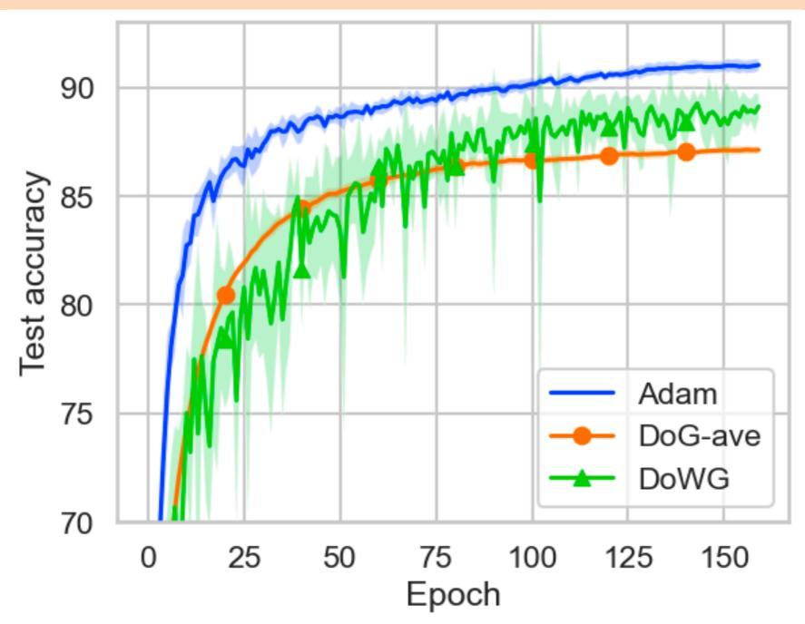
Test accuracy, VGG11 on CIFAR10. Unstable behaviour. Coordinate-wise estimation doesn't work.
